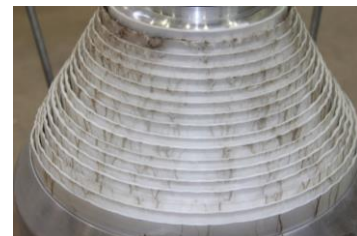
Fig. 2. Flashover traces on a peaking capacitor.
