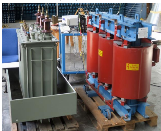
Fig. 1. DUT's: Oil-insulated medium-voltage transformer T1 (left) and resin-insulated medium-voltage transformer T2 (right)
