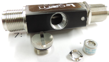
Fig. 1. Example of a GDT surge protector (taken apart).
