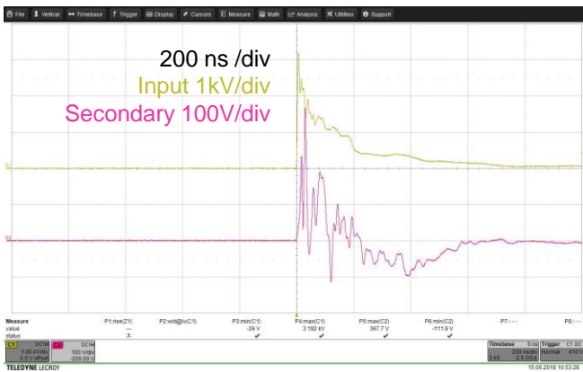
Fig. 7. Fast Input pulse (green) and voltage on secondary side (purple)
