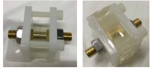
Fig. 4 SiC-PCSS packaged epoxy
