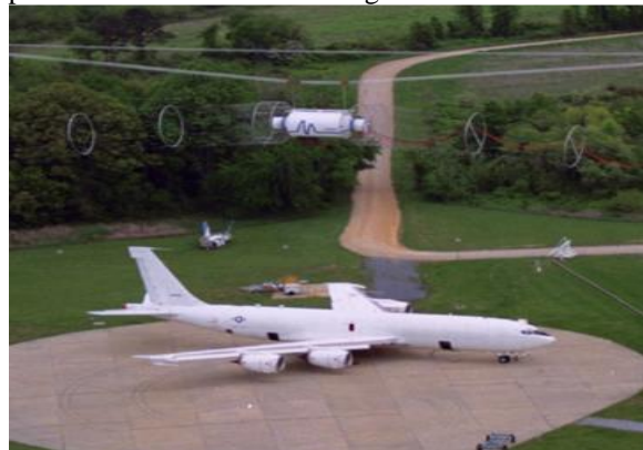
Figure 15 Aircraft electromagnetic pulse test
